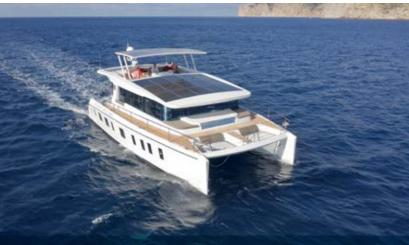
The **SILENT 55** is an oceangoing catamaran that meets the highest ship building standards, respects the environment and makes no compromises regarding luxury cruising at the same time. This yacht is powered by solar energy. In the standard configuration the two electric 30 kW motors achieve a maximum speed of 12 knots.
